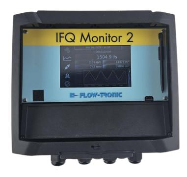
The IFQ MONITOR 2 is a user-friendly monitor, data logger and converter for Flow-Tronic flow sensors. It is equipped with one RS485 digital serial communication port for **RAVEN-EYE® 2(+), BELUGA, BELUGA A/V or PHOENIX 2** flow sensors and one 4-20 mA input for external level.
